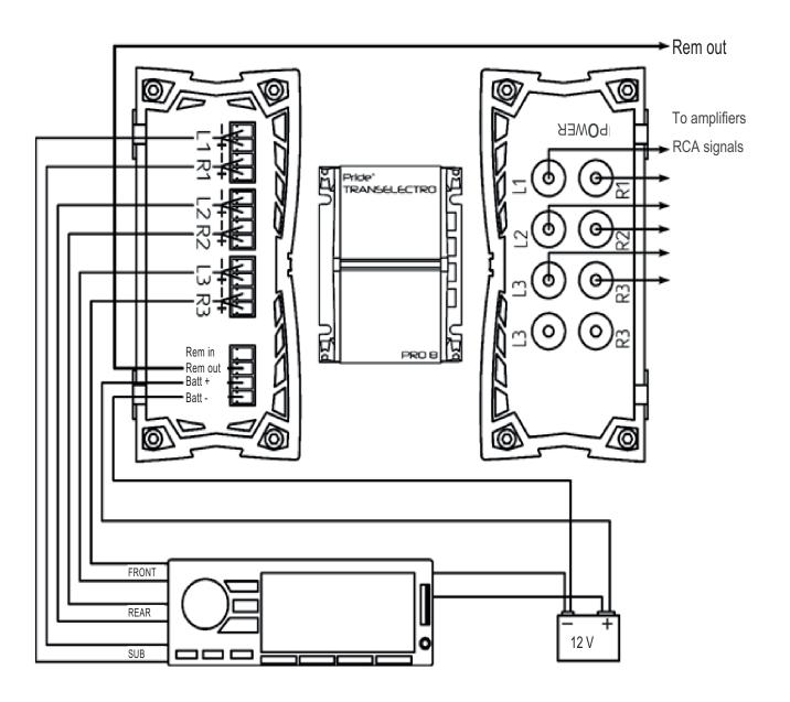
Typical wiring diagram. The REM IN pin is left unconnected by default.
